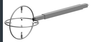
The 'Vxsp' style Ultrasonic Anemometer is a 3 axis, 3d, 15 cm, scientific Ultrasonic Anemometer This design incorporates a full circle on both axes which strengthens the arms for more durability. Like the "Vx" probe, it is designed for flux measurements in plant and forest canopies where wind speeds are extremely low, and directions are highly unpredictable.
